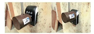
► IK08 test Architect<sup>®</sup> ARC-B reader with keypad is rated IK08. Test report no. 145623-697063.
