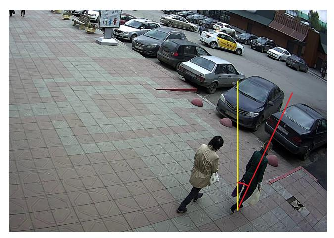
The camera must be placed almost horizontally: the tilt angle of the camera in relation to the ground must not exceed 30 degrees.
